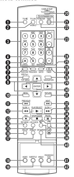
Buttons with a small dot on the left side of the name can also be used to operate your TV. (LF pg. 86)
